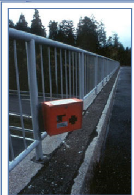
Figure 2. Infrared still camera setup with protective case on Slovenian bridge.
