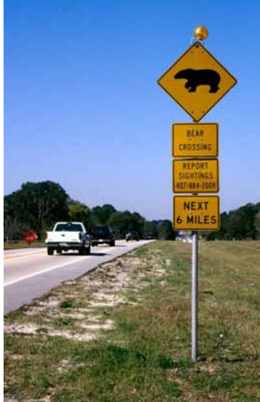
Figure ES17. Photo. Permanently flashing Florida black bear warning signs in the Ocala National Forest, FL (copyright: Marcel Huijser).
