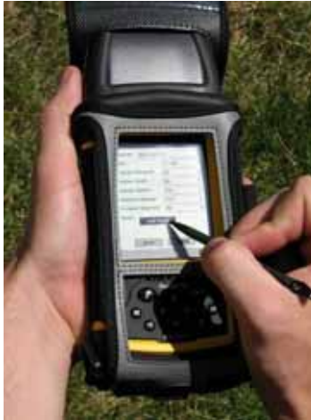
Figure ES18. Photo. Roadkill observation collection system (ROCS), a GPS-enabled PDA for animal carcass data collection (copyright: Amanda Hardy, WTI).
