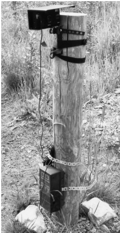
FIGURE 6 Infrared camera set-up in Banff National Park to monitor use of structures.
